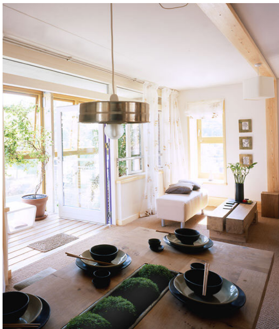
Room exposed thermal mass with sunspace
