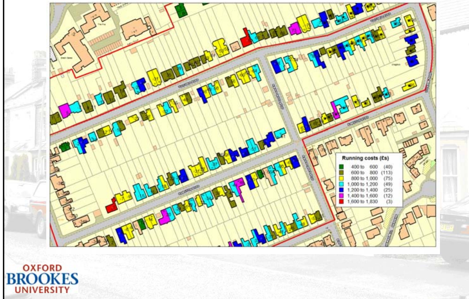
Thematic map of dwellings in the case study showing annual fuel costs
