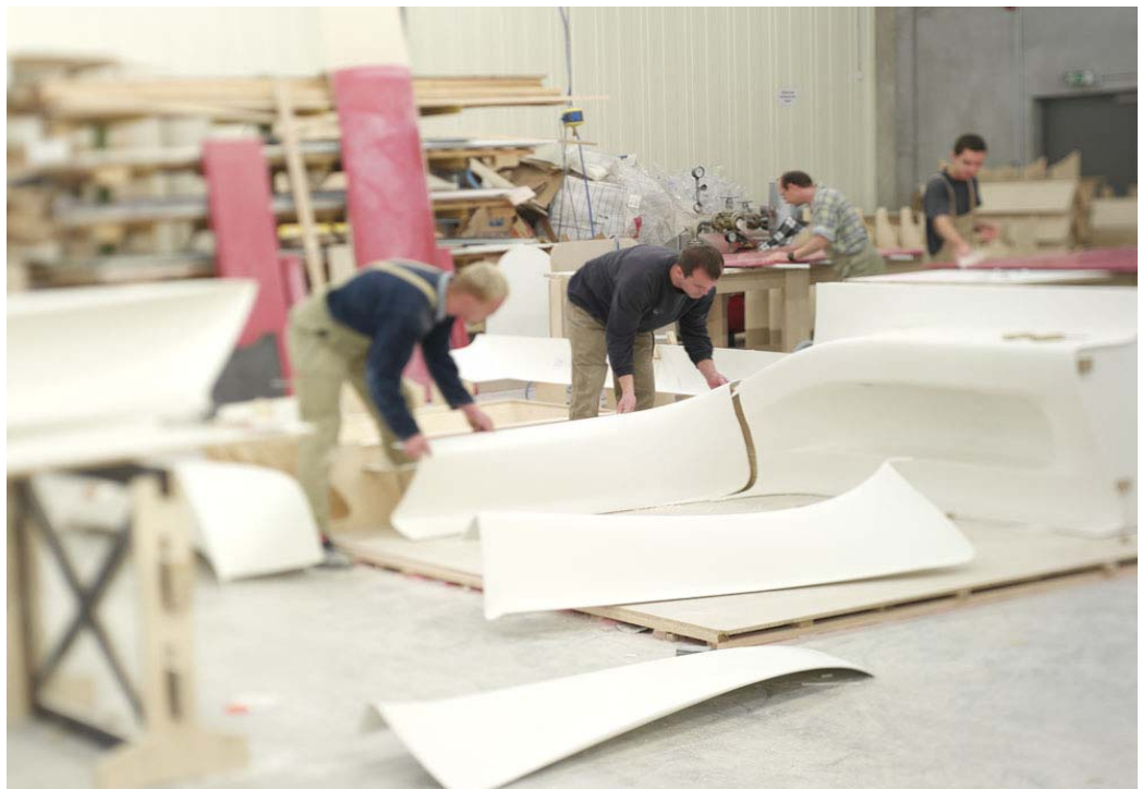
Illustration 12: putting together the bed frame
