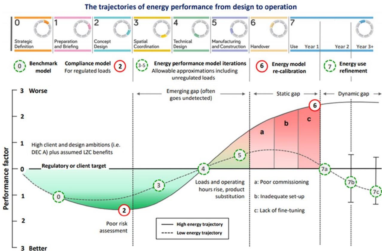
Figure 3: Two trajectories of emerging energy performance during procurement: a ‘performance gap’ trajectory, and a Soft Landings trajectory with periodic modelling and improvement interventions. (Diagram ©Dr Roderic Bunn. Published in CIBSE TM62: *Operational performance of non-domestic buildings: Occupant satisfaction and GDPR good practice guide*. 2020. Chartered Institution of Building Services Engineers. London.
