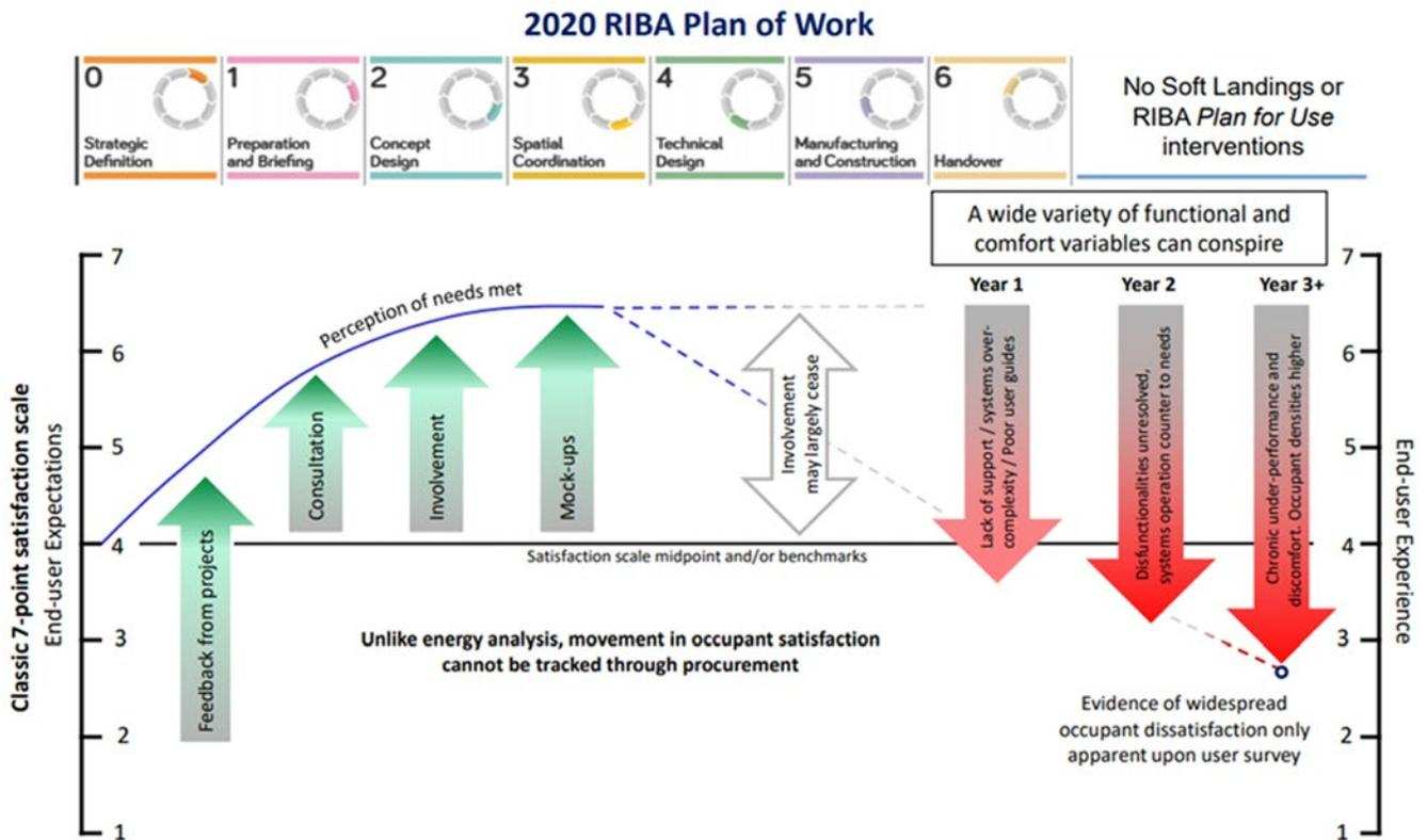
Figure 4: Occupant dissatisfaction can emerge from occupant surveys, despite architects' best efforts during early design consultations. (©Dr Roderic Bunn. Published in CIBSE TM62: *Operational performance of non-domestic buildings: Occupant satisfaction and GDPR good practice guide*. 2020. Chartered Institution of Building Services Engineers. London.
