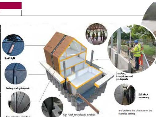
The concrete ring beam is cast adjacent to the structure and retains the amount of debris entering the dock. Some siltation is inevitable, so the base is profiled to create a void under the house, which can be flushed out from time to time.
