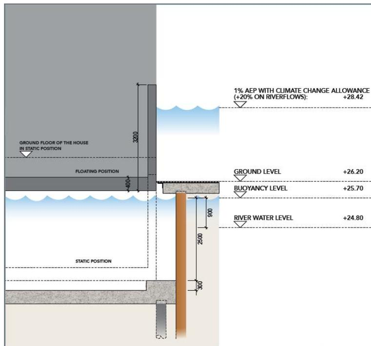
**b.** The 'can-float' base functions similarly to the hull of a ship. It provides the building's buoyancy and supports the structural frame of the dwelling. The 'can-float' hull (shown in Figure 3.15) is formed from reinforced waterproof concrete to protect against water ingress. The foundation is designed to be heavy enough to prevent crabbing and impact damage, but sufficient in volume and light enough in mass to provide buoyancy.
