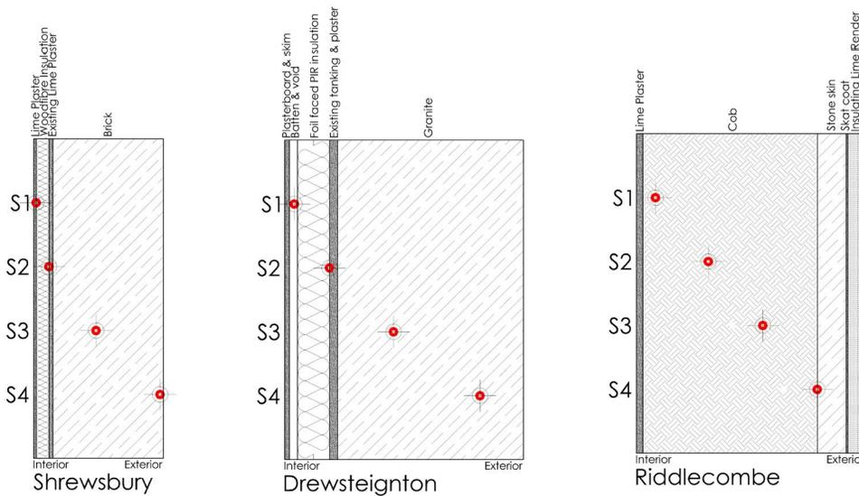
Figure 1 Locations of interstitial hydrothermal gradient sensors in walls at Shrewsbury, Drewsteignton and Riddlecombe, SPAB Building Performance
