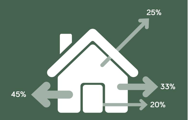
45% heat loss through uninsulated solid walls 33% heat loss through uninsulated walls 25% heat loss through the loft/roof space 20% heat loss through windows & doors
